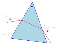
• As prism rotates about light's entrance point,  $\delta = 2(\varphi + \psi - \alpha)$  decreases, reaches minimum  $\delta_M$ , then increases
