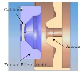
developing a new technique to design electron guns that produce these beams. The students were provided the required specifications for a device to drive the TEVATRON accelerator at Fermi National Laboratory.
